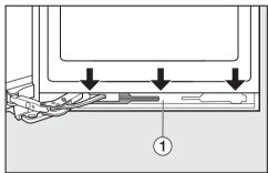
Remove panel ① from the soft-close mechanism and ease it off carefully from above bit by bit. Take care not to damage the door seal.
